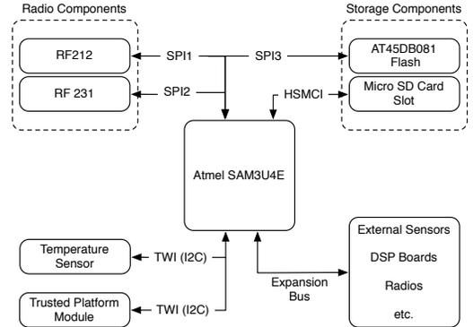
Fig. 1. Functional diagram of the major Opal components.
