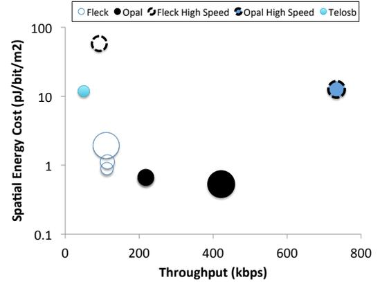
Fig. 3. Comparison of the spatial energy cost versus throughput of TelosB, Iris\* and Opal. The Iris\* and Opal results show single and dual radio results, as well as a high throughput scenario of 1000 kbps transmissions with a single radio. The size of bubbles indicates the absolute power consumption for high rate transmissions.
